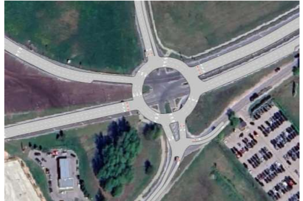
Figure 36 – Improvement of the P133/Dzirnietu Intersection (from Current Situation to Alternative 2) Source: Ineco
