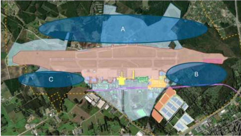
Figure 4 – Terminal and Apron Alternatives Source: Ineco
