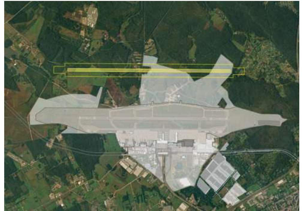
Figure 76 – Independent parallel Runway System Source: Ineco
