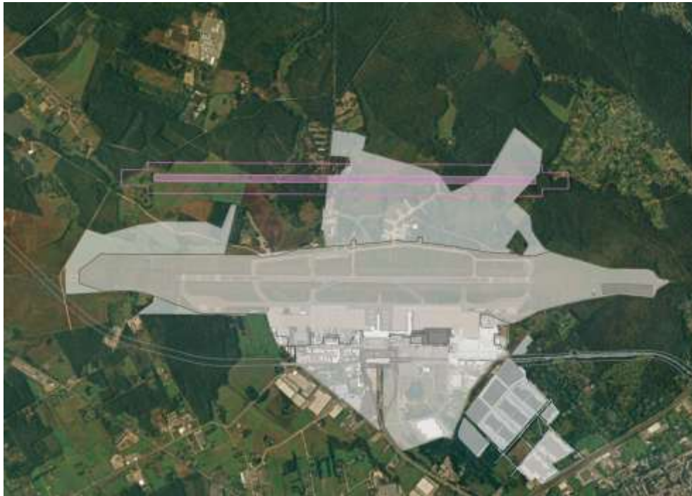
Figure 75 – Dependent parallel Runway System Source: Ineco
