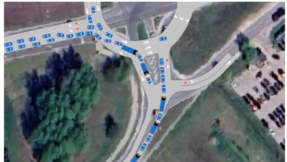
Figure 18 – Traffic simulation – 2050 – Possible critical point Source: Ineco
