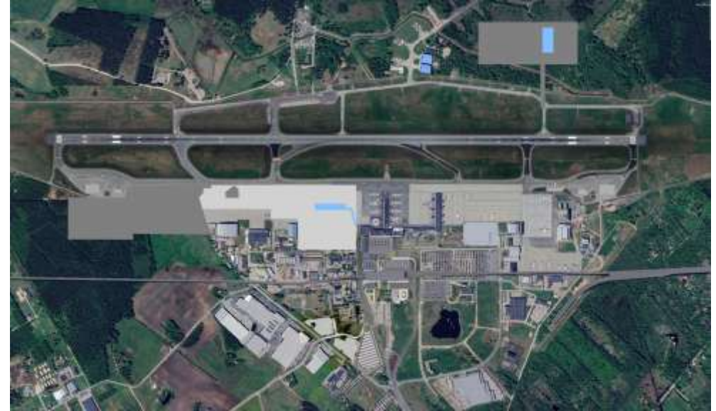
Figure 9 – Terminal and Apron Alternative 5 – South Double-sided Perpendicular Pier Source: Ineco
